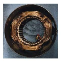
When balanced three-phase voltage is applied to the windings of the stator, the balanced three-phase currents flows in three interconnected phase windings. These currents produce a magnetic field which results in torque to turn the rotor. *In the most common type of electric motor, AC induction, electric power is not conducted to the rotor directly, but*
