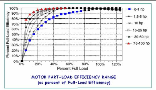
Efficiency values at partial load points are also tabulated below for energy-efficient and standard motor models of various sizes.
