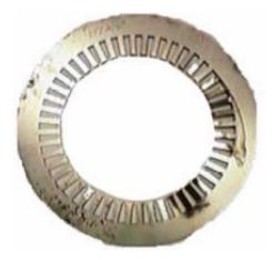
Insulation is inserted to line the slots, and then coils wound with many turns of wire are inserted into the slots to form a circuit.
