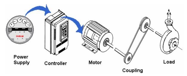
Each component of this system can be optimized for reliability and efficiency.
